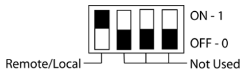
Figure 3-7. SGI 4-pin Configuration Switch for Ethernet
